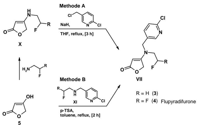
**Figure 5.** General synthetic pathways to butenolides (VII) by the methods A and B.
